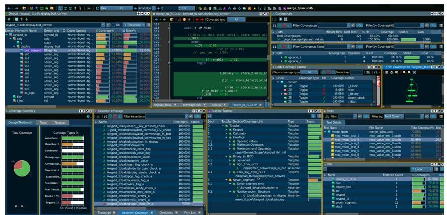
Questa One Sim also integrates VHDL into its industry-best constraint solver, allowing it to generate more complex VHDL constrained random stimulus. It also enables the ability to save the VHDL functional coverage data into the Unified Coverage Data Base format, offering VHDL verification as a native part of Questa One Sim. UVM already incorporates these new features to enhance the already popular VHDL verification methodology.
